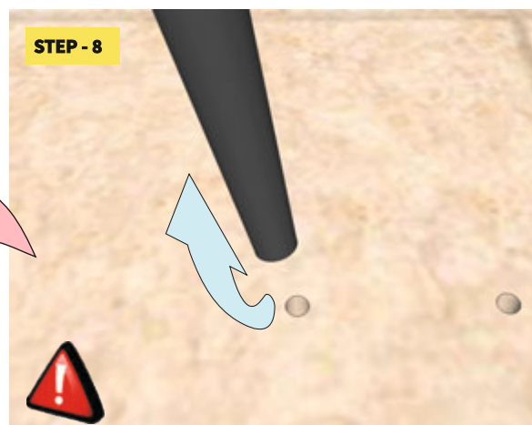
STEP - 8 Not cleaned dirt may cause decrease strength of this joint!
