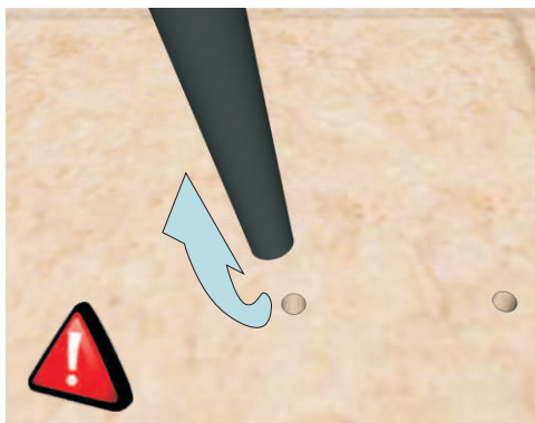
Not cleaned dirt may cause decrease strength of this joint!
